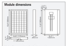
Hole diameter 0.26 inch (6.6 mm) Mounting hole dimensions are center to center
